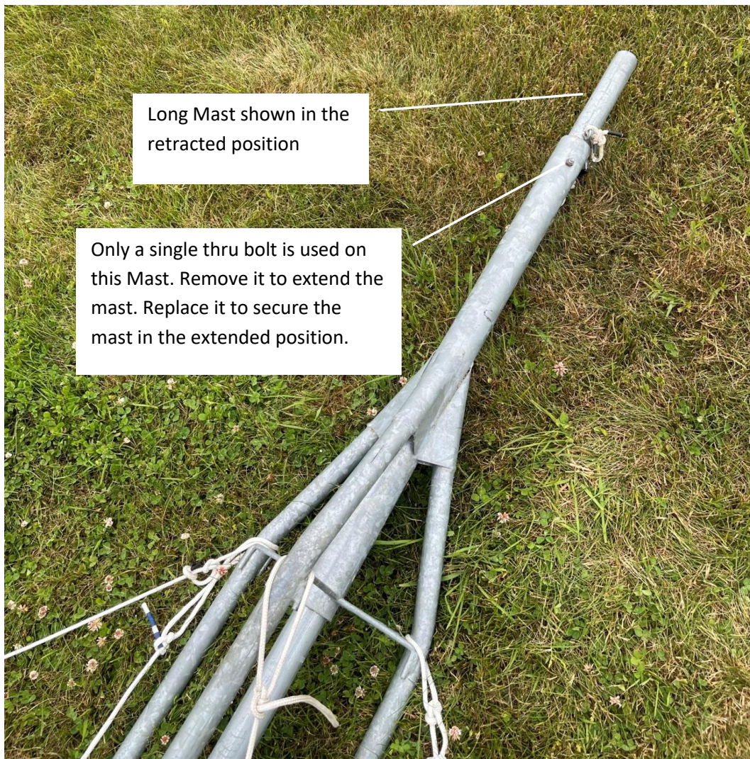
Figure 8 Long Mast stored in Retracted Position: This Long Mast is stored in the retracted Position and uses only one thru bolt to secure it in the extended position
