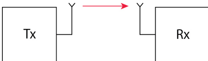
Figure 1: Example of SISO system, where one antenna is used on each side of the RF link.
