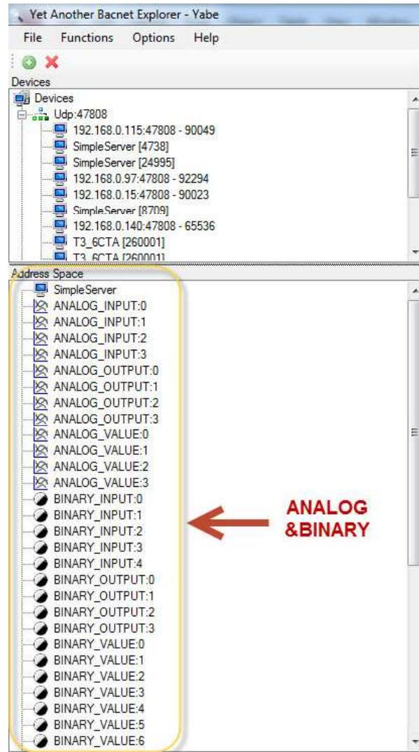
Step4.In the “Address Space” tab,click the “ANALOG\_VALUE”,it will show the information of “log ANALOG\_VALUE”in the BacnetProperty tab. And it ‘s the same with “ANALOG\_OUTPUT” and other items.
