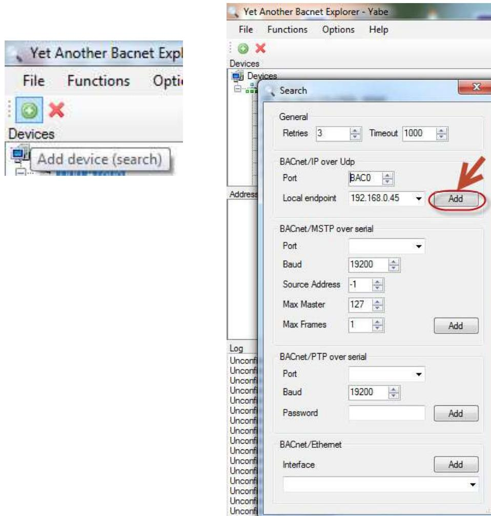
Step3. You can find your device IP as below. Double click the left mouse button, you can find your device and the bacnet information in the "Address Space" tab.
