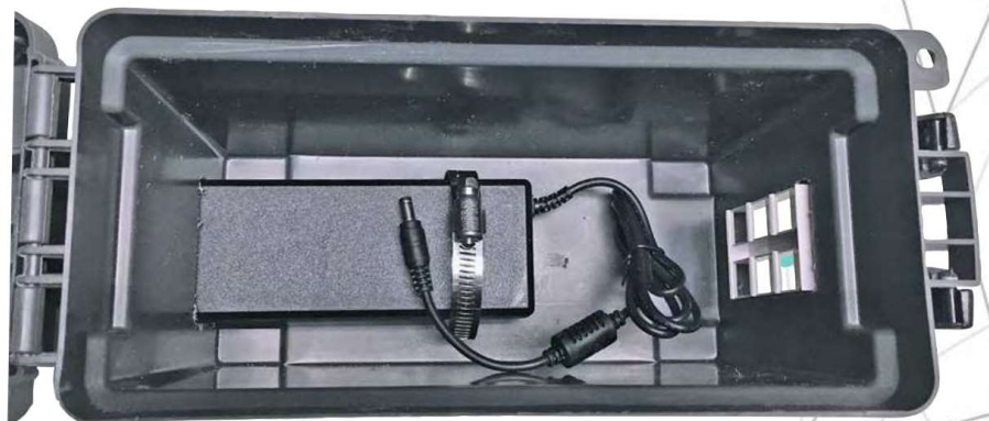
Figure 2 — For a secure base, install the power supply through a hole on the bottom of the box with a hose clamp. Notice that the data jack plate is installed.
