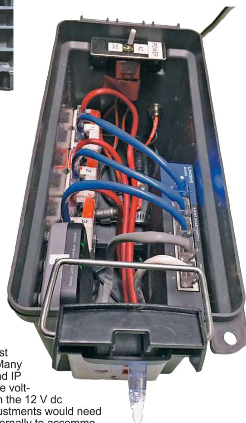
Figure 3 — The red cables are for the POE injectors and the blue cables are for the data connections. Note that there are port numbers on the hardware.
