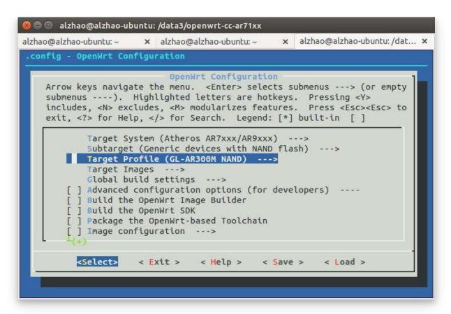
The make process will takes around 1 hour for the first time because it needs to download a lot of data from t he Internet. After compiling finished, you will find the following firmware files in bin/ar71xx/
