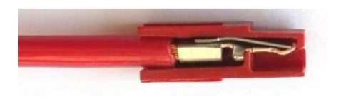
The Contact fits through the gap between the housing and spring and is inserted until the contact "snaps" over the end of the spring
